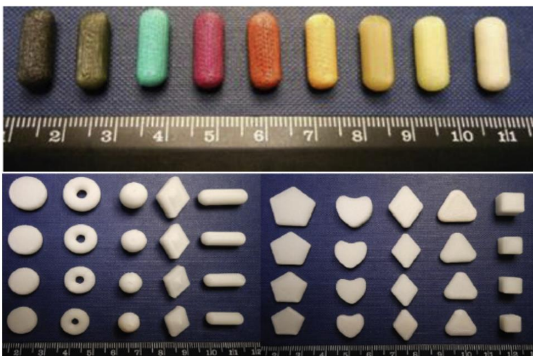
Figure 18. (A) Capsule-shaped printlets in different colours and printlets with different geometries (disc, torus, sphere, titled diamond, capsule, pentagon, heart, diamond, triangle and cube) presented in four different sizes (125).
